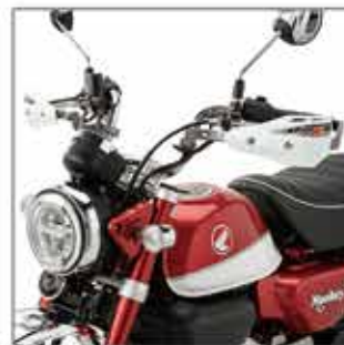
All of the optional armor hand guard protector series (P.52) can be installed. (The image is equipped with ZETA X2 protector)
