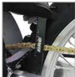
Can be used as gauge for chain play.
